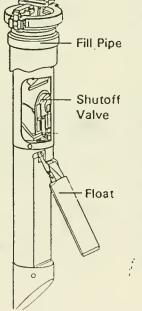
Some automatic shutoff devices work in two stages. The first stage drastically reduces the flow of product to alert the driver that the tank is nearly full. The driver can then close the delivery value and still have room in the tank for the product left in the delivery hose.
